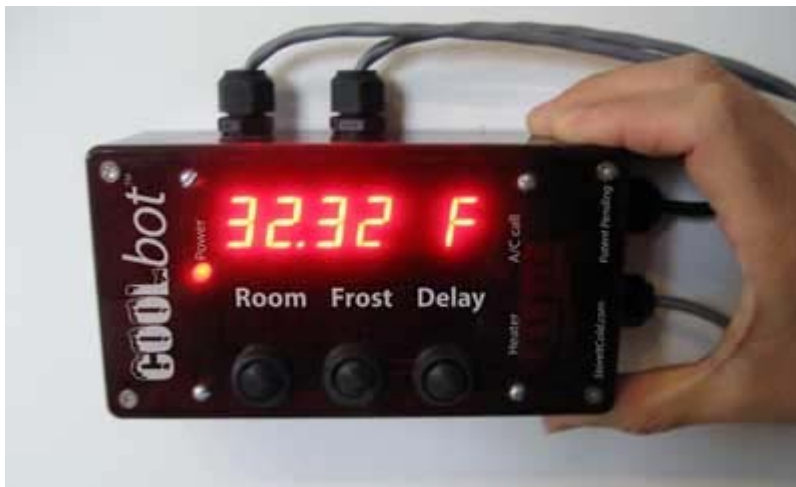
Figure 1. Photo of COOLbot™ Controller
